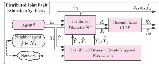
Fig. 1. Distributed Joint Fault Estimation Procedure
