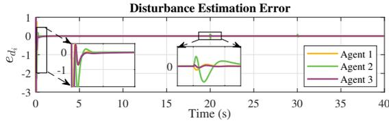
Fig. 6. Disturbance estimation error,  $e_{d_i} = d_i - \hat{d}_i, i = 1, 2, 3$
