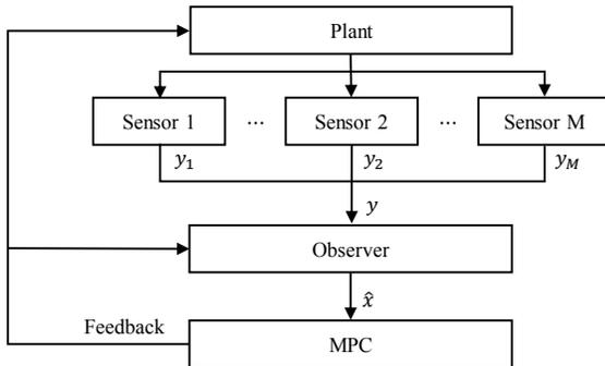
Fig. 1: Output feedback MPC with centralized estimation
