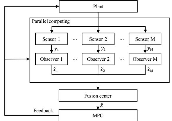
Fig. 2: Fusion-based output feedback MPC
