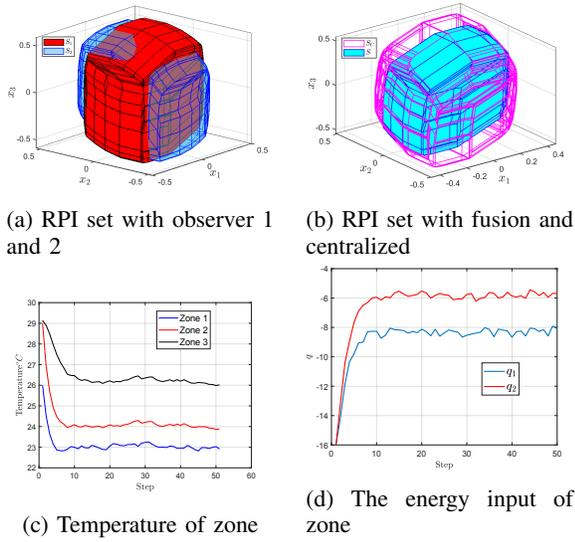
Fig. 3: Invariant sets under different control strategies and the temperatures of with the controller:  $S_c$  denotes the tube for ROFMPC with centralized estimation.
