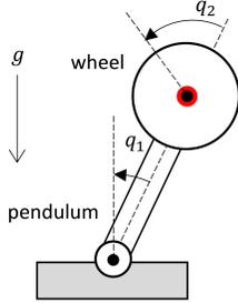
Fig. 1. Schematic of inertia-wheel pendulum system.
