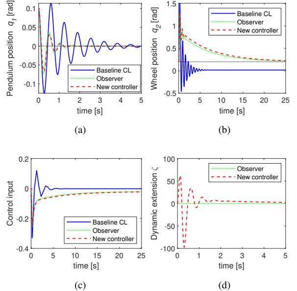
Fig. 3. Simulation results for IWP with position-dependent matched disturbance  $\delta_1 = -0.1$  and  $G^\top h(q) = q_2$ : (a) pendulum position; (b) wheel position; (c) control input; (d) dynamic extension  $\zeta$ .
