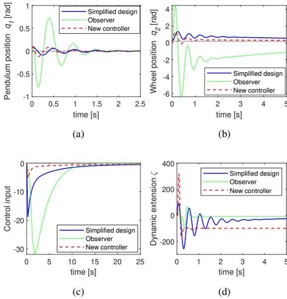
Fig. 4. Simulation results for IWP with position-dependent matched disturbance  $\delta_1 = -10$  and  $G^T h(q) = q_2^2$ : (a) pendulum position; (b) wheel position; (c) control input; (d) dynamic extension  $\zeta$ . “Simplified design” refers to the controller (18) which assumes  $G^T h(q) = 1$  and  $\partial_q \Psi = 0$ .
