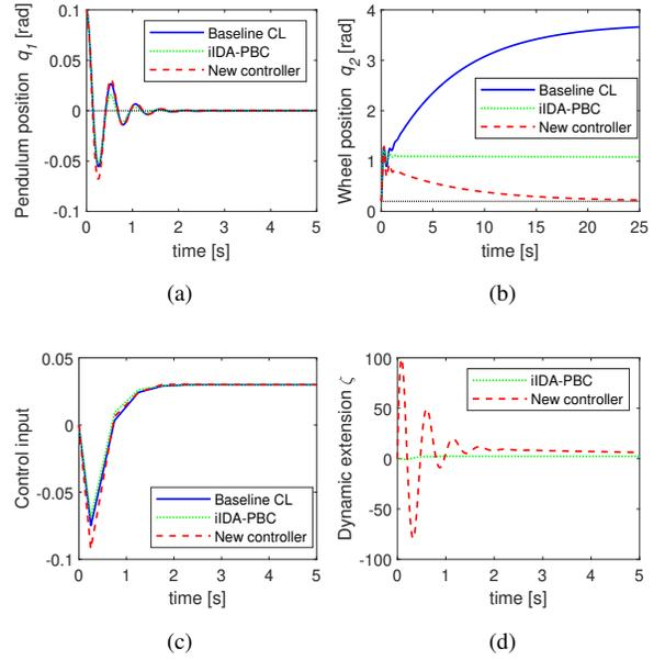
Fig. 2. Simulation results for IWP with constant matched disturbance  $\delta_1 = 0.03$  and  $G^\top h(q) = 1$ : (a) pendulum position; (b) wheel position; (c) control input; (d) dynamic extension  $\zeta$ .
