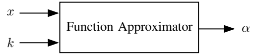
Fig. 1. The function approximator takes as input the state and time step, then outputs a reach probability value of satisfying the reach specification.
