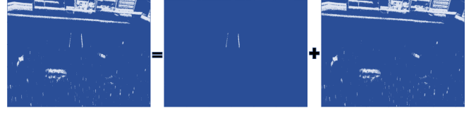
Fig. 2: Monochromatic images generated using state-of-the-art event-based cameras. The full image I to the left can be decomposed into one that contains only the runway image I_r (center) and the remaining objects/noise I_n (right), i.e., I = I_r + I_n .
