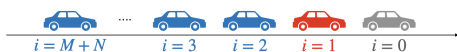
Fig. 1. The mixed-autonomy platoon considered in the experiments. The gray vehicle is the leader, followed by an AV (red), followed by several HVs (blue).
