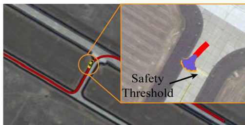
Fig. 4. Our algorithm is applied to assure safety in potential runway incursion scenarios. Once the ground vehicle is determined to have crossed a designated safety threshold, the aircraft is cleared to land. timestep set would inhibit any progress regardless of the relative size of later timesteps' sets.
