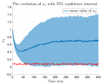
Fig. 3. Trajectories of x_3 by PI Algorithm 2 with chance constraints. The shaded area represents a 75% confidence interval for 500 independent experiments. The red dotted line denotes the time-varying safety constraints.
