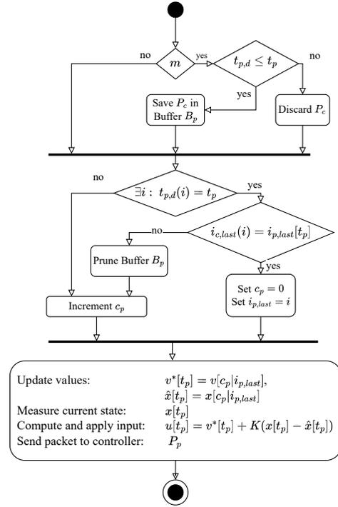
Fig. 2. Plant side algorithm. The top part handles incoming control packets, the middle part checks on prediction consistency, the bottom task computes and executes the control input.
