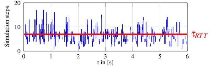
Fig. 6. Round trip time of the balance robot example. Everything above  $\bar{\tau}_{RTT}$  as well as all steps where the line is broken is considered as a dropout.
