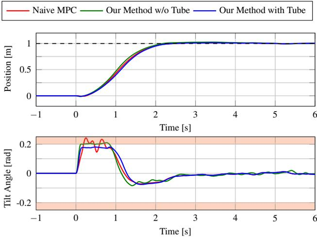
Fig. 5. Position and tilt angle of the balance robot. We compare a nominal MPC with the tube-based MPC method.
