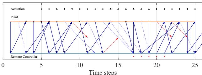
Fig. 8. Network behavior of the CSTR simulation. Dashed lines show dropped (red) and discarded (blue) packets. The geometric symbols (circles, triangles, diamonds) denote, which packet was used for the corresponding actuation. As expected, the distance from the appearance of the symbol on the plant line to its time of application on the actuation line is  $\bar{\tau}_{RTT} = 4$ . Red crosses on the bottom indicate the recovery mode at the remote controller.
