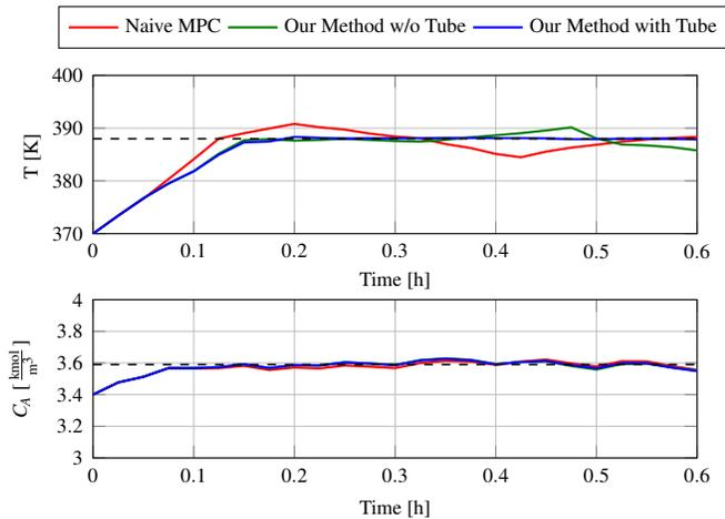
Fig. 7. State development over time for the CSTR simulation. The top depicts the temperature  $T$ , concentration  $C_A$  is shown on the bottom.
