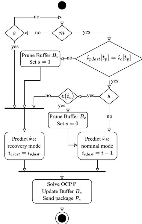
Fig. 3. Remote controller algorithm. The top part describes checks for measurement and prediction consistency, the middle part determines the state prediction, and the bottom part solves the OCP.
