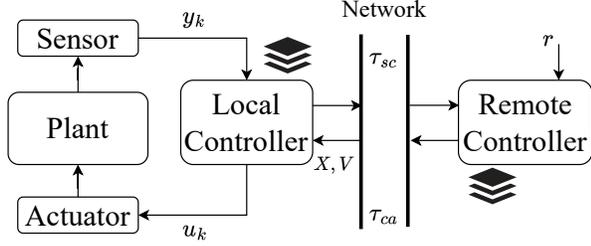
Fig. 1. Considered setup. The local controller forwards measurements to the remote side and receives actuation signals from the remote controller over a lossy network.
