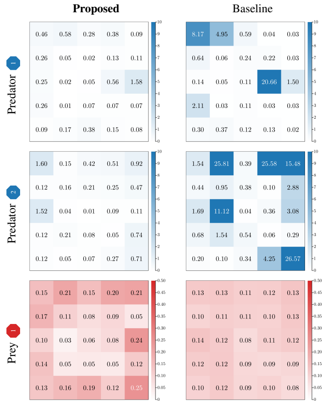
Fig. 3: Heatmaps showing Kullback–Leibler divergence D_{KL}(\Pi_s^i \parallel \hat{\Pi}_s^i) between the equilibrium policy \Pi_s^i and the observed policy \hat{\Pi}_s^i at each state s in the GridWorld for all three players. All values rounded to two decimal places, the smaller (lighter color) the better.
