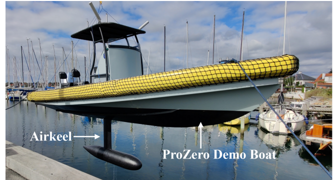
Fig. 1. Photographic view of the ProZero Demo boat equipped with the novel Airkeel mechanism (Courtesy: Dacoma ApS and ProZero, Tuco Marine Group)
