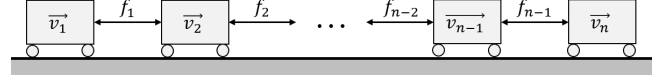
Fig. 3. Vehicle platoon model of n cars where the direction of travel is to the right.
