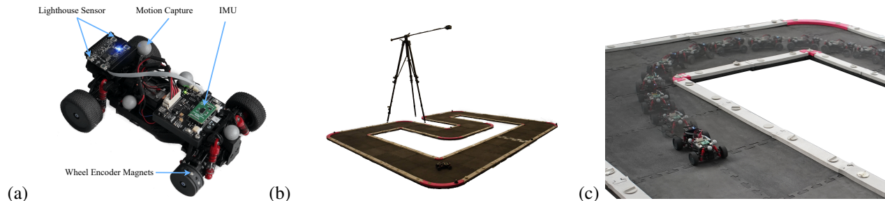
Fig. 1: (a) Chronos car based on a Kyosho AWD buggy model with custom electronics: IMU, wheel encoders with magnets in wheels, and Lighthouse positioning deck. (b) Track setup with Lighthouse base station. (c) Hardware experiment.
