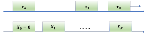
Fig. 1: The first illustration shows the position and direction of the vehicles. The second illustration depicts the relative position X_n = x_0 - x_n .
