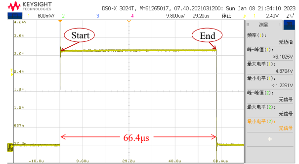
Fig. 4. The total computation latency of the Algorithm 2 on the STM32F407 @168MHz with N_p = 6 and N_c = 4 .
