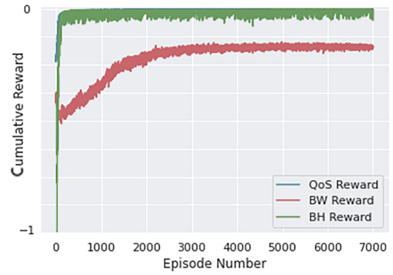
Fig. 6: Discounted cumulative reward for QoS metric, BW consumption and BH load obtained by MO-A2C . Rewards related to BW consumption and BH load are multiplied by 10 and 0.1, respectively.
