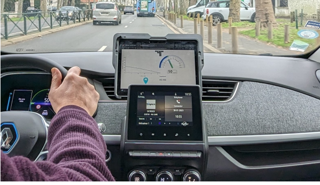
Fig. 1: The tablet mounted on the dashboard displays the ED target speed.
